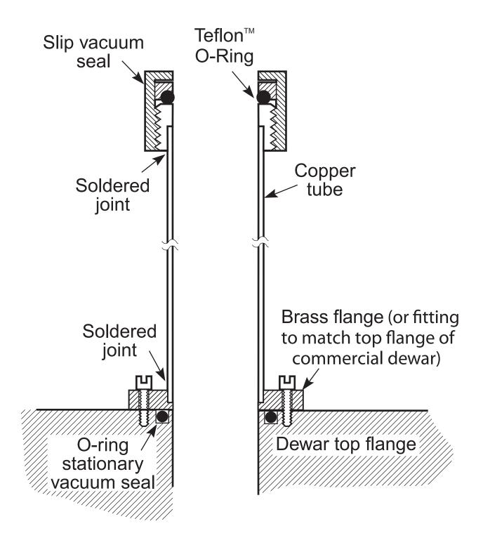
FIG. 1.9 Warming chamber, into which the sample holder of Fig. 1.6 can be withdrawn at the end of a test to prevent condensation of water on the cold sample surface.
